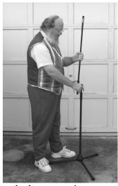
To set up, open the tripod feet of the stand, point the boom section upward, and secure it. Extend the extension pole to its full length, inside the curtain, and tighten it. Place the "T" joint on the end of the boom. Extend the mike stand upward until the curtain is just off the ground and tighten the mike stand.
